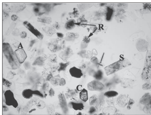
Fig. 7. Microphotograph of 0.063–0.125 mm fraction separated from smectite clay, Struganik quarry, western Serbia. A — Apatite; R — Radiolarians; S — Spongi spicules, and C — Zircon.
