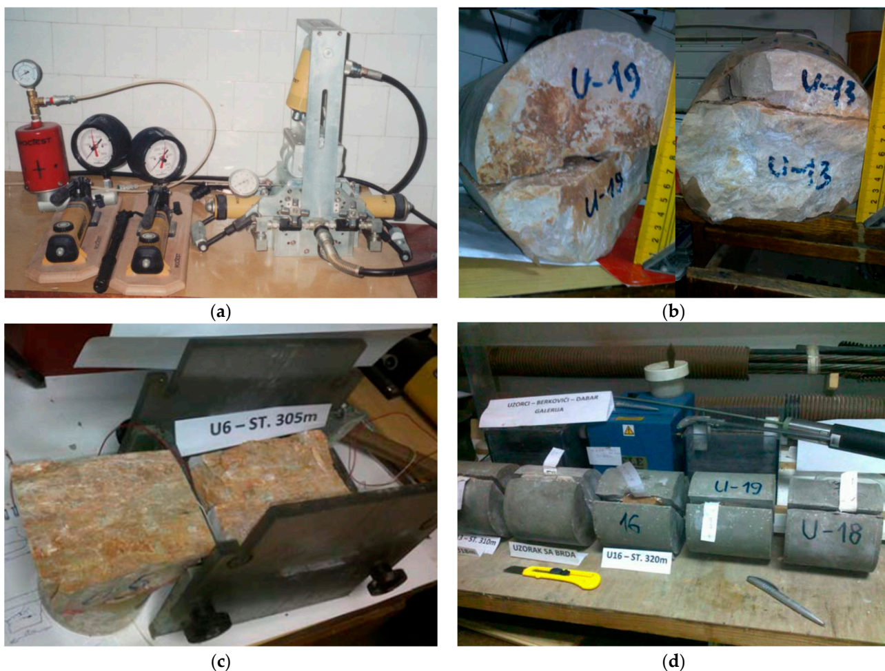
Figure 5. Procedure for shear testing along discontinuities: (a) shear device used for testing; (b) engineering–geological inspection and evaluation of joint samples; (c) placing of samples in mould prior to cementing; and (d) cemented samples prepared for testing [28].
