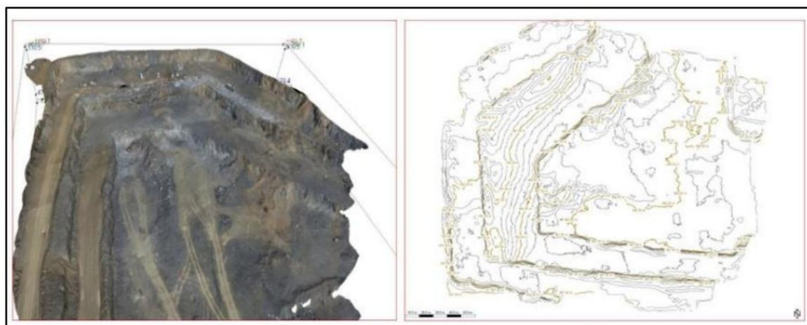
**Figure 5-** 3D image of terrain (left) with contour plot isoline (right) obtained by UAV (3gsm gmbh, 2019)
