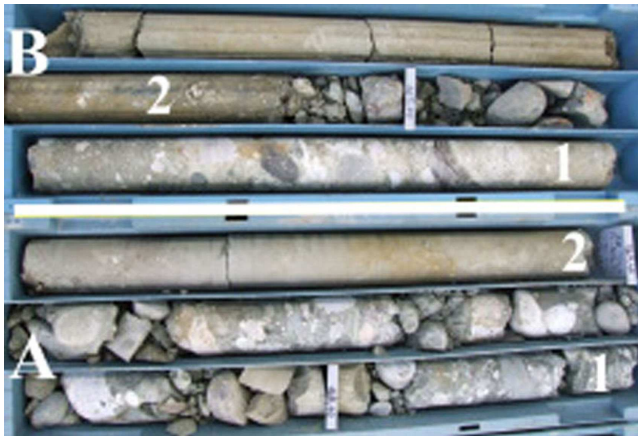
Fig. 8. Close-up view on the two clastic sequences (A, B). 1, Gravel; 2, Sand (RTK-1501, 108-110 m).
