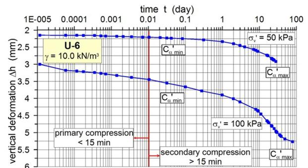
Figure 6. Compressibility diagram for loading level  $\sigma'_1 = 50$  and 100 kPa (samples of series B)
