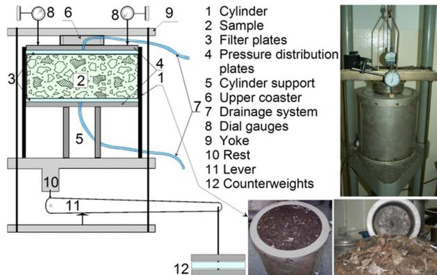
Figure 3. Construction of oedometer apparatus
