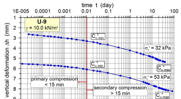
Figure 7. Compressibility diagram for loading level  $\sigma'_1 = 32$  and 53 kPa (samples of series C)
