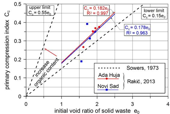
Figure 10. Relationship of the primary compression index and initial void ratio
