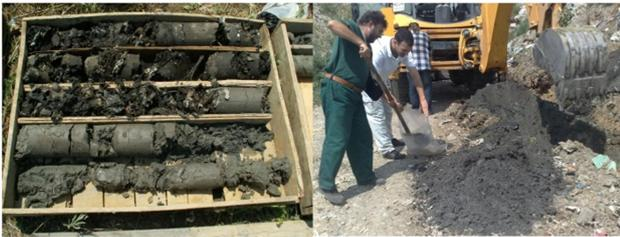
Figure 1. Analysed municipal waste from exploration boreholes and exploration pits.
