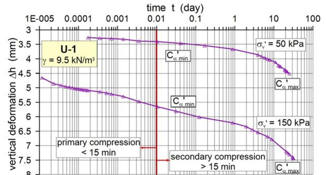
Figure 5. Compressibility diagram for loading level  $\sigma'_1 = 50$  and 150 kPa (samples of series A)
