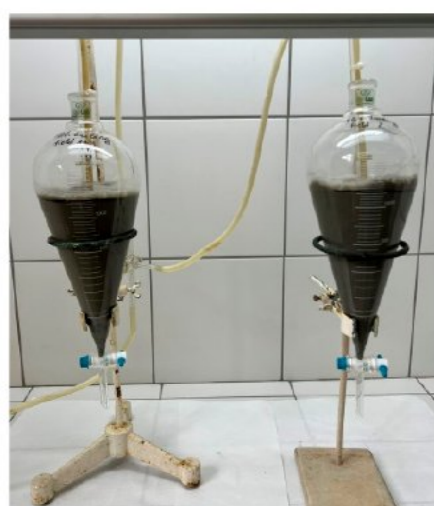
Figure 1. Separatory funnels for ozone leaching of Composite I and Composite II samples.
