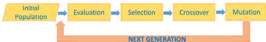
Figure 2. The basic flowchart of genetic algorithm [50].
