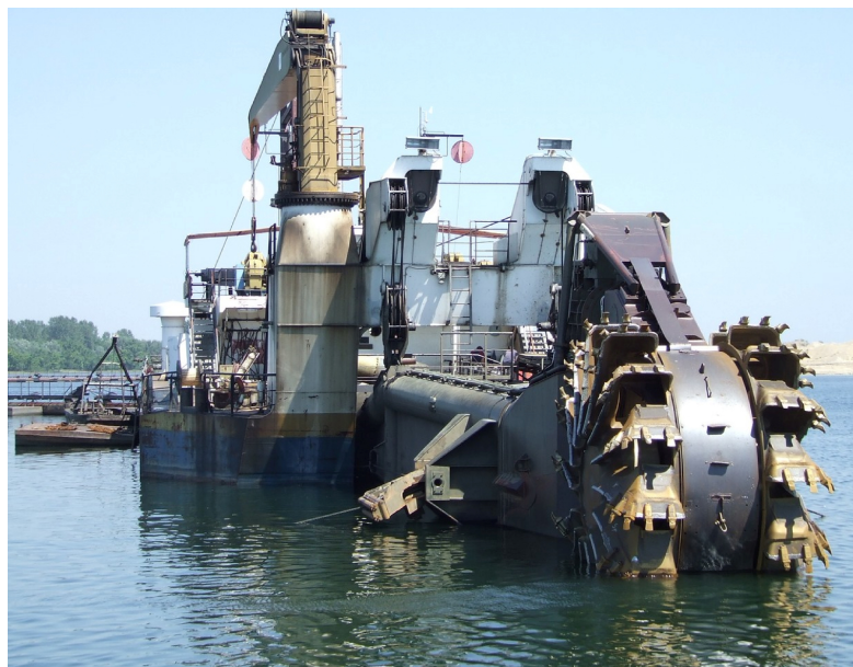
Figure 3. Bucket-wheel dredger “Kovin I” with bucket wheel type UCW-450 [19].
