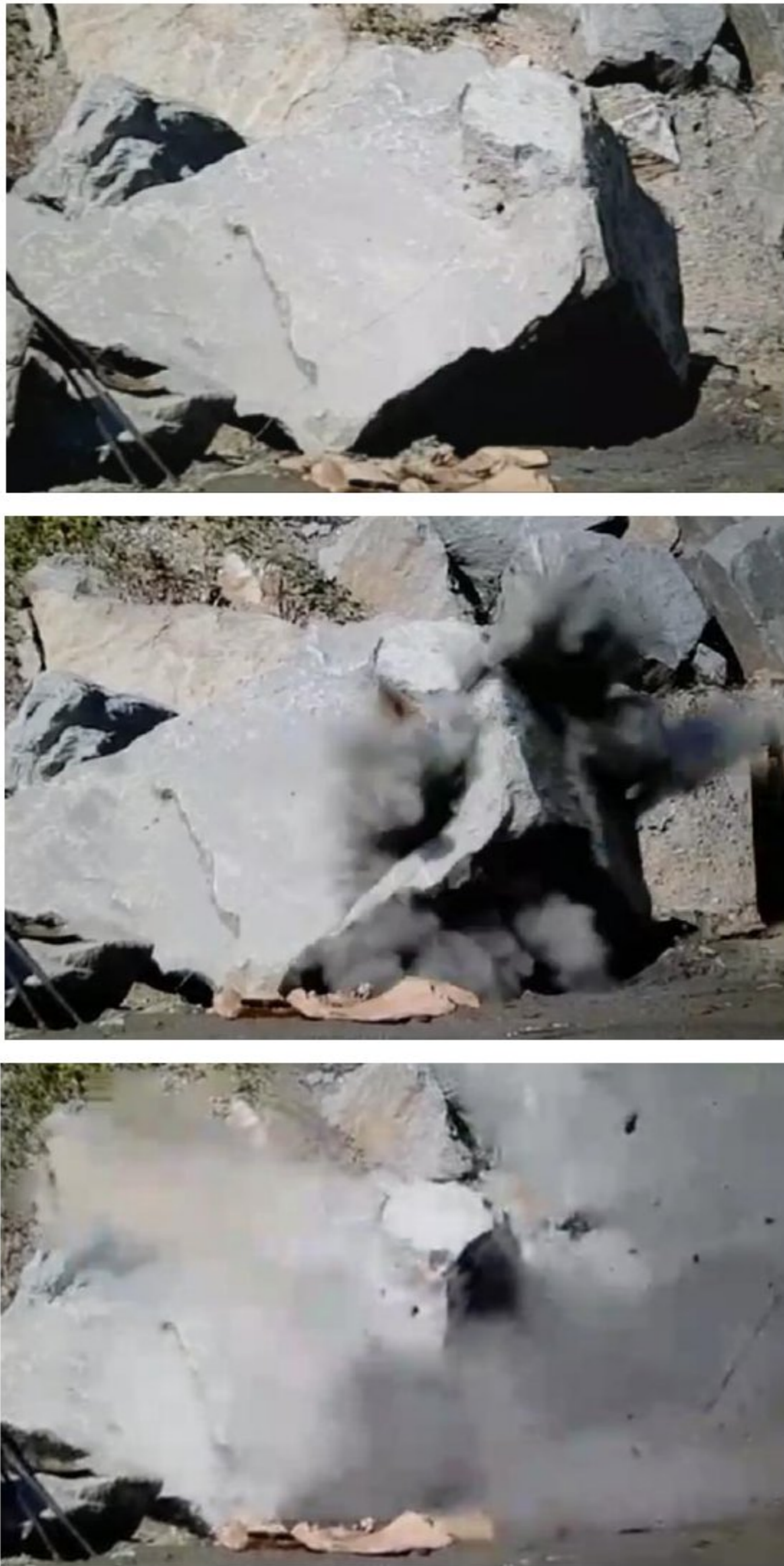
Fig. 6 The results of polygon test of non-detonating chemical mixture [2,6]
