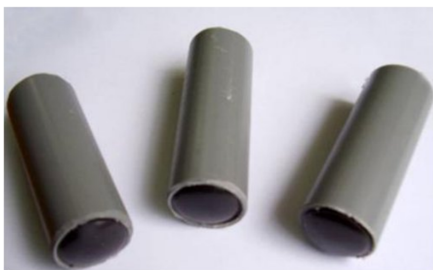
Fig. 2 Cartridges charged with non-detonating chemical mixture [2,6]
