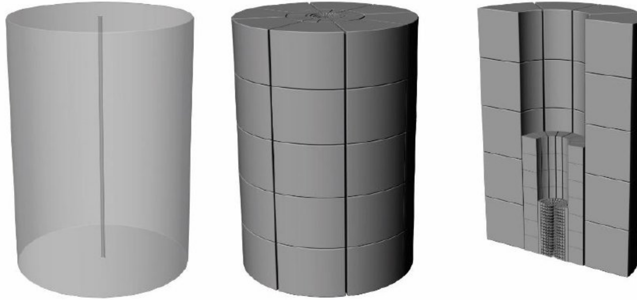
Figure 6 3D illustration of specimen fragmenting
